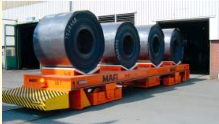
Bumpers for material flow system for coils
