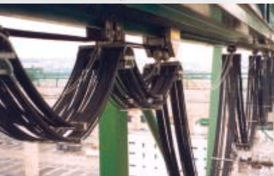
Energy and data lines on a container crane
