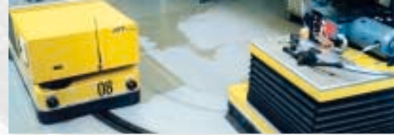
Floor conveyor system featuring inductive power transfer
