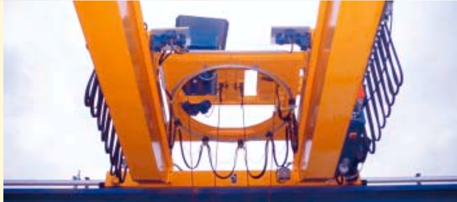
Flexible energy supply for straight and circular paths
