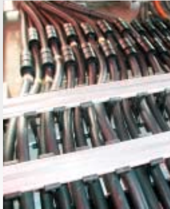
Cable for energy guiding chains with clips for strain relief
