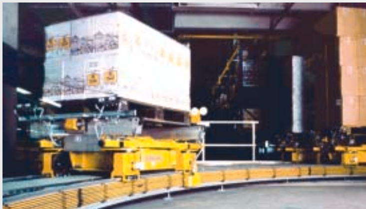
Transfer car used in the food industry with Powertrans® Ib data transmission
