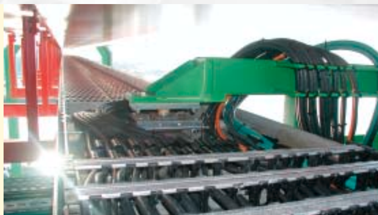
Energy guiding chain designed for long travel distance on a ship-to-shore container crane
