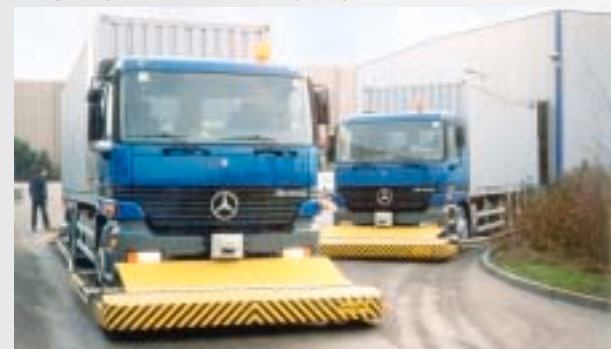
Safety bumpers for driverless transport system
